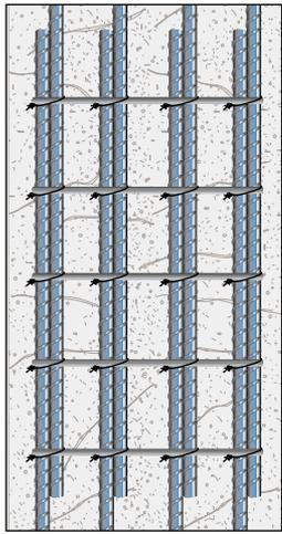
*Lap splices depend on concrete for strength, and therefore lack structural integrity and continuity in concrete construction.*
